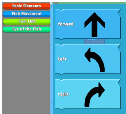
Figure 19: The blocks for the forward movement, turn left and turn right.
