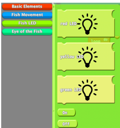
Figure 20: The blocks to control the single color LED.
